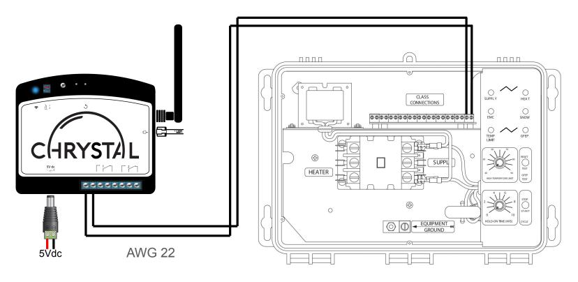
Note: In this configuration when CHRYSTAL stops it's command, it activates the melt time configured in the APS controller, therefore we recommend reducing the melt time to a minimum when a Preheating monitoring plan is selected
