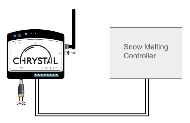
If the primary controller receives commands by means of a dry contact then Chrystal will be compatible.
