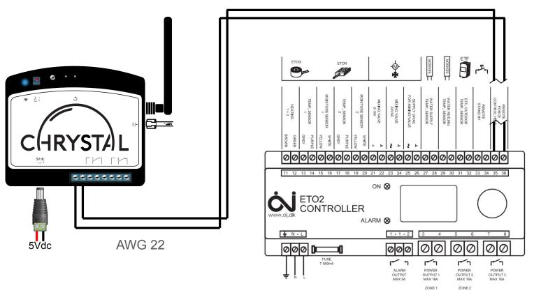
Note: In this configuration when CHRYSTAL stops it's command, it activates the after run time configured in the ETO2 controller, therefore we recommend reducing the melt time to a minimum when a Preheating monitoring plan is selected
