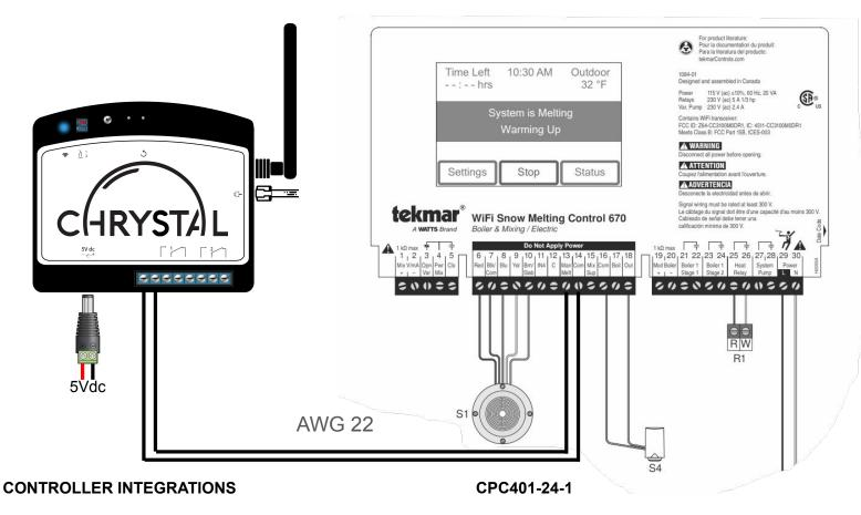
Note: With Hydronic systems, the purpose of this connection it to replace idling and reduce operating costs. When CHRYSTAL is connected, idle mode is set to the lowest allowable temperature.
