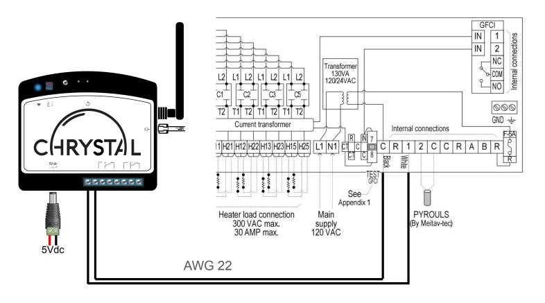
Note: In this configuration when CHRYSTAL stops it's command, it activates the melt time configured in the Meitavtech controller, therefore we recommend reducing the melt time to a minimum when a Preheating monitoring plan is selected
